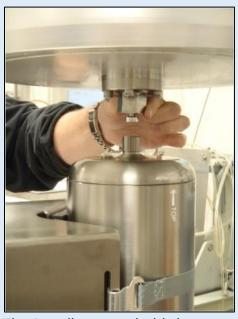
The installer must hold the nut manually while guiding the shaft into position.
